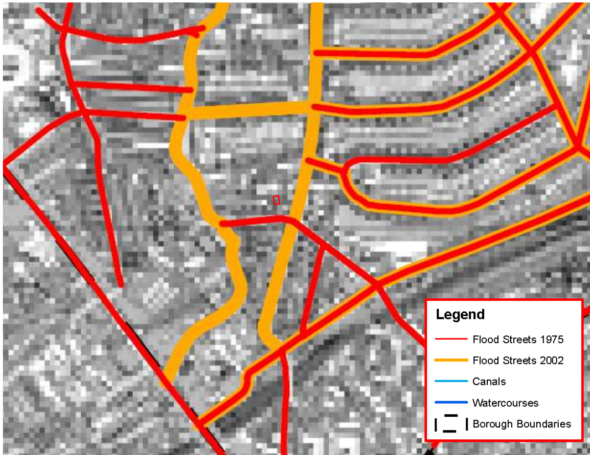
Figure 3 Camden surface water flooding (taken from SFRA Appendix A Map 22)
