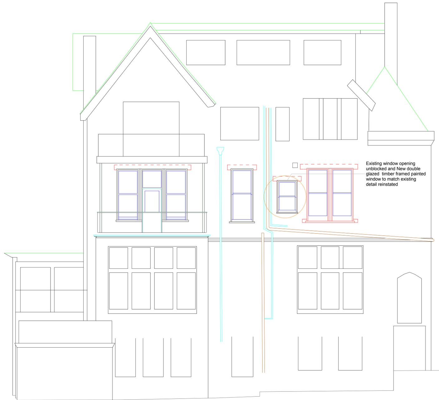
Existing window opening unblocked and New double glazed timber framed painted window to match existing detail reinstated
