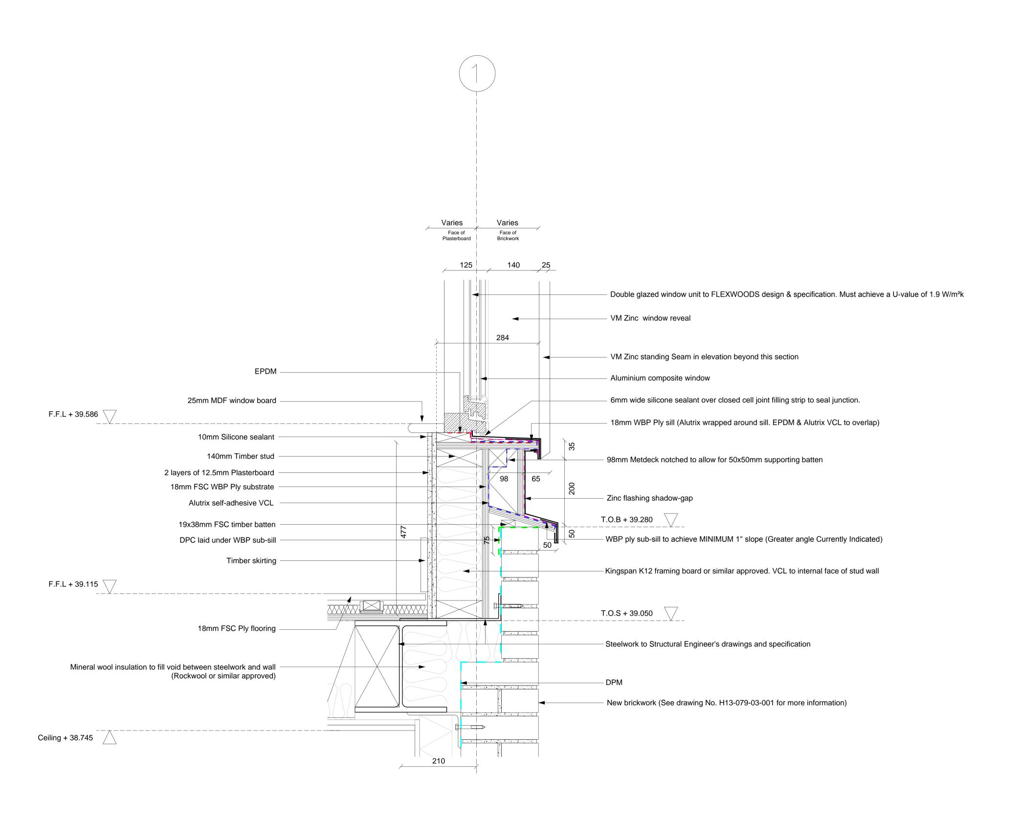
Junction Between Zinc Cladding and Existing Brick Wall Detail
