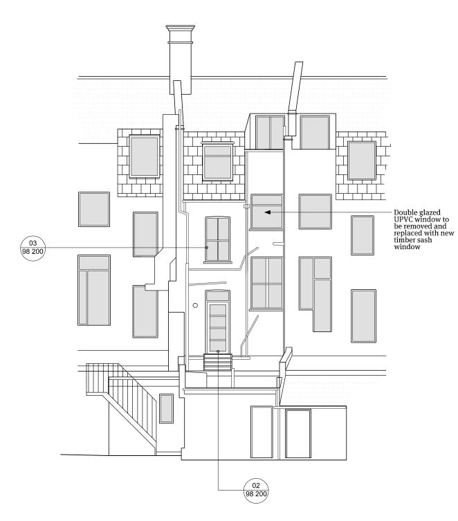
$01\frac{\text{Existing Front Elevation}}{_{1:100@\text{A}3}}$
