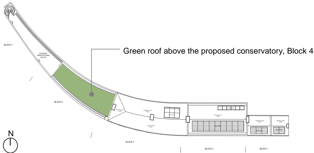
Figure 3.10: Proposed roof plan for the Fish & Coal Offices showing the proposed location of the green roof.
