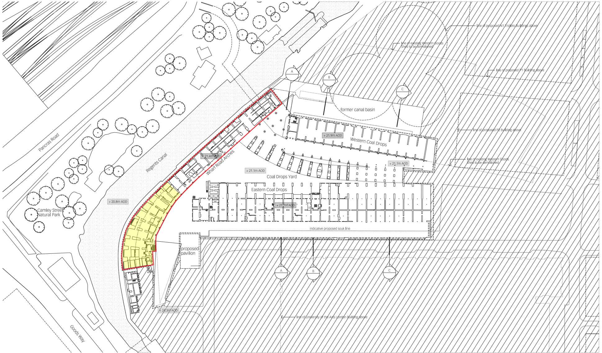
Figure 2: Lower level plan of viaduct arches - yellow area denotes first area to be refurbished
