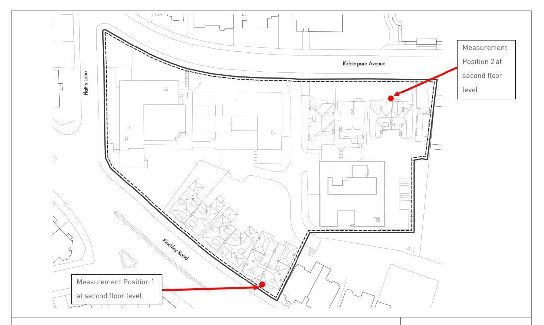
Site Plan Showing Measurement Positions at second floor level
