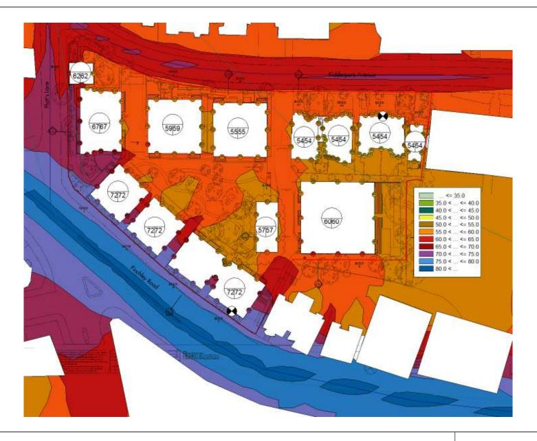
CadnaA Noise Map showing daytime  $L_{eq,16hour}$  noise levels at 1.5m and maximum façade incident  $L_{eq,16hour}$  noise levels.
