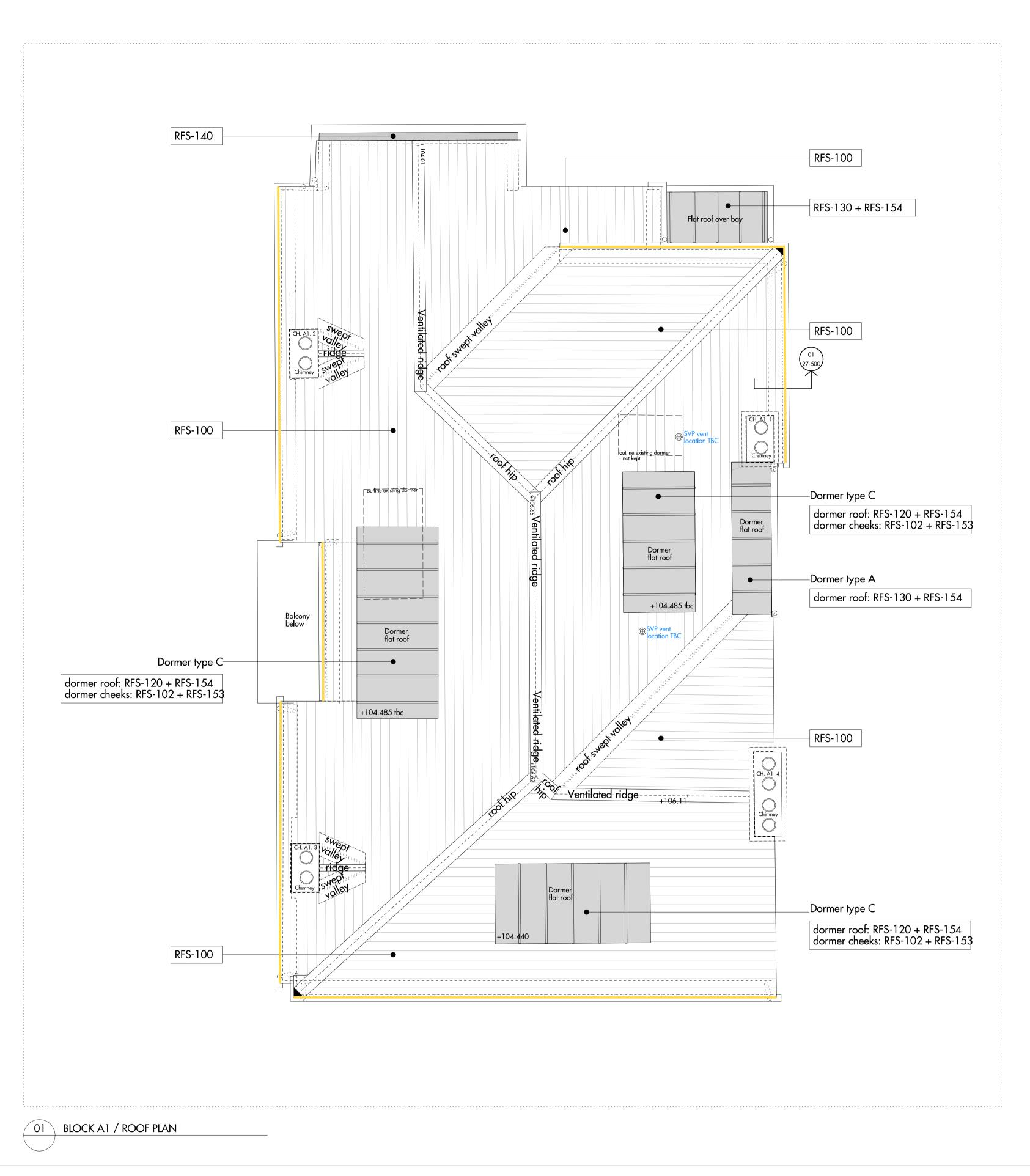
EAVE TYPES: Eave Detail Type A Eave Detail Type B Eave Detail Type C Eave Detail Type D ventilated ridge: half-round clay ridge tile with ventilation system roof hip: bonnet clay tiles roof hip end tile: arris type clay tile - TBC roof swept valley: round valley clay tile
