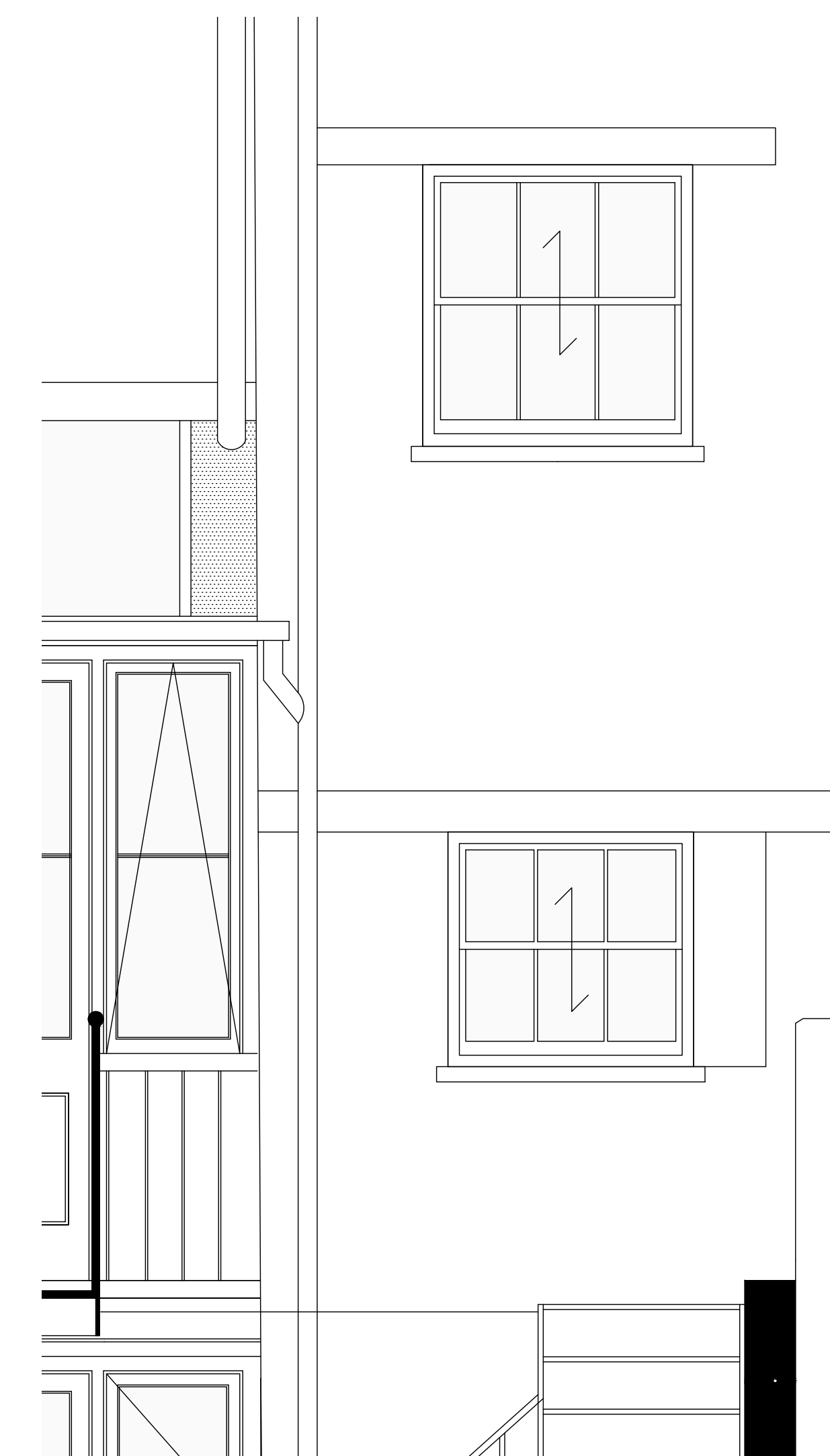
Above: new sash windows to rear elevation (ground floor and first floor RH)
