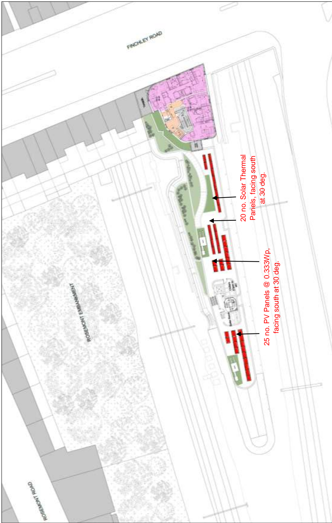
Figure 14: Proposed Third Floor Roof Plan with PV Layout
