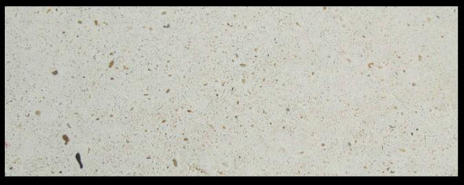
Leigh Street: Cast Stone Cast stone to all sills, soffits and stone facades with an aggregate mix of wet-cast concrete mix of Cotswold gravel and a 50%:50% mix of Cotswold and Dolomite sands and white cement with an acid etched surface finish with a light grey mortar ( Euromix M3WLK34).
