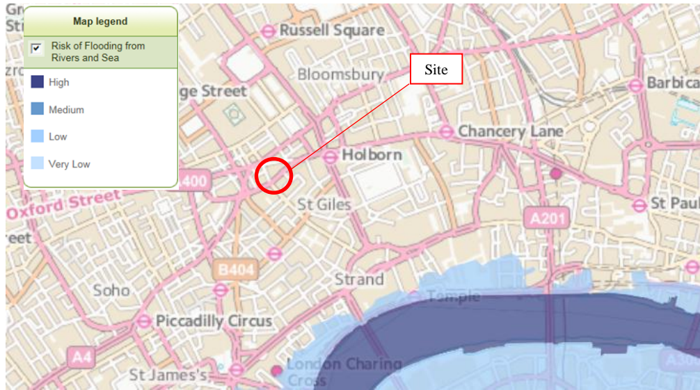
Figure 4 – Risk of flooding from River and Sea
