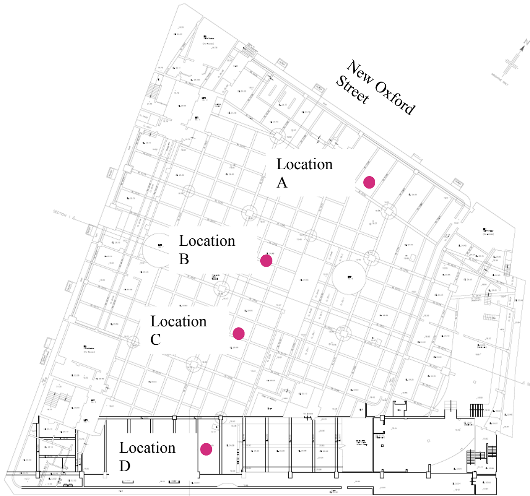
Figure 2: Groundborne noise measurement locations
