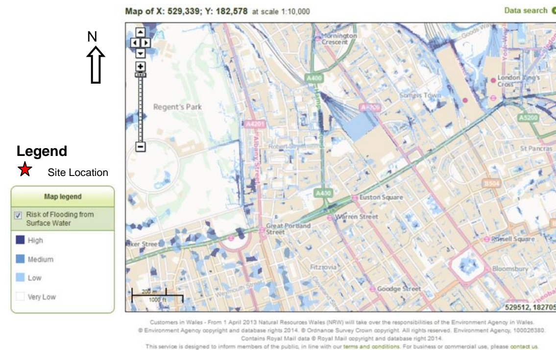
Figure (n) Flooding from Surface Water (Extract from Environment Agency flood map)
