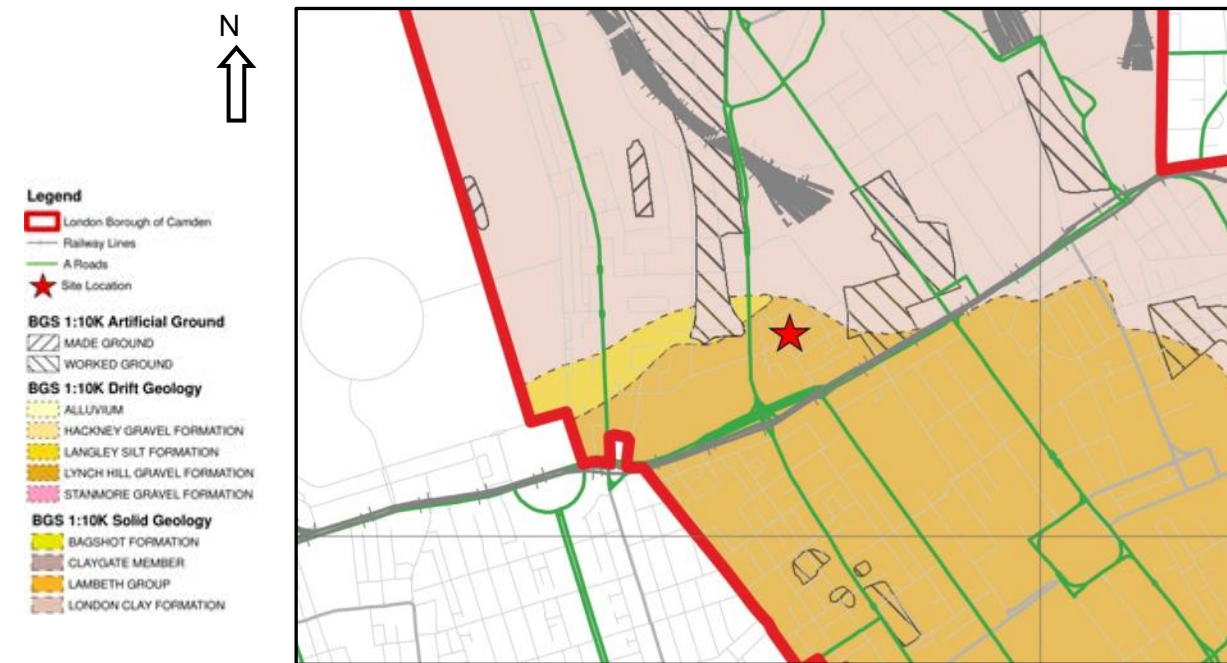
Figure (e) Geological Map (Extract from Fig 4 of Camden Geological, Hydrogeological and Hydrological Study)
