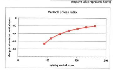
CONSOLIDATION SETTLEMENT beneath a flexible rectangular loaded area
