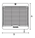
Window fixing hole Ø 184mm
