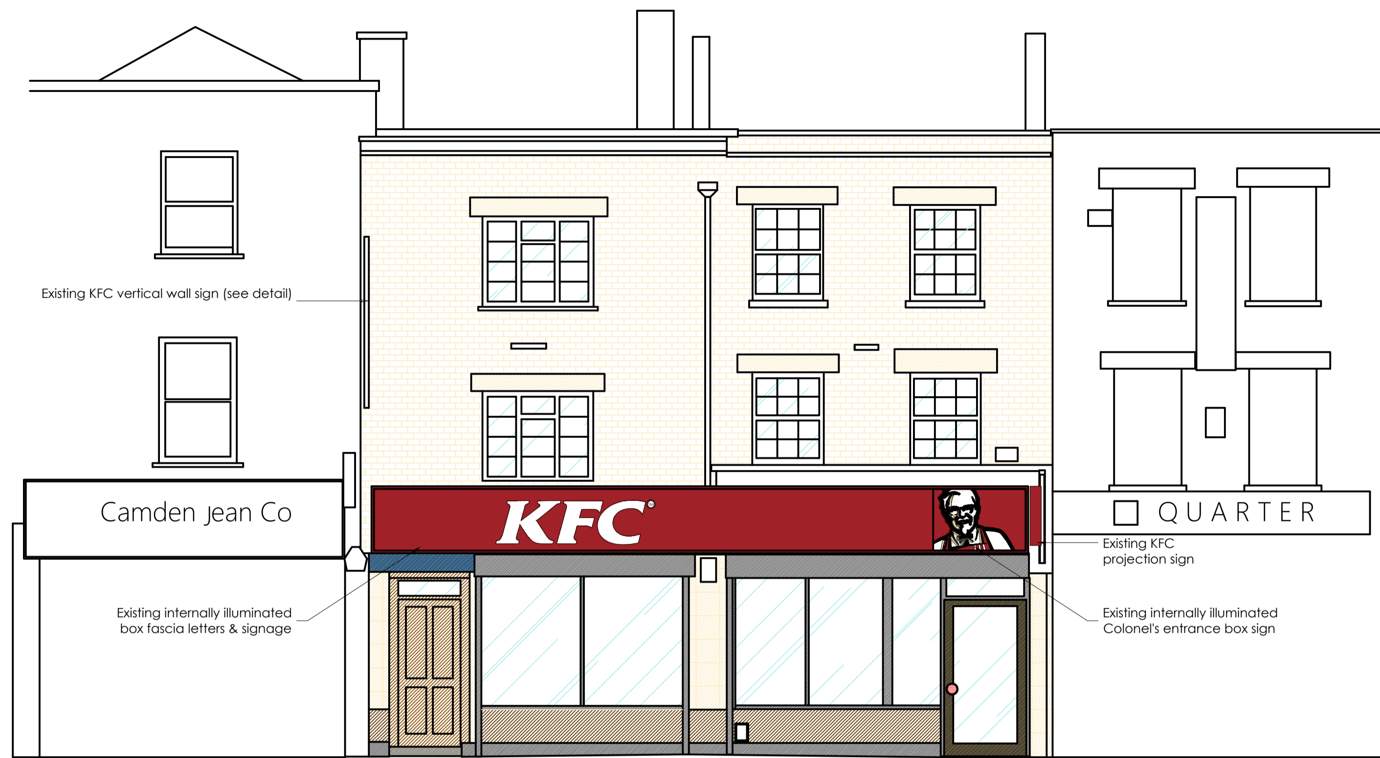
existing shopfront elevation scale - 1:50 @ A1 / 1:100 @ A3
