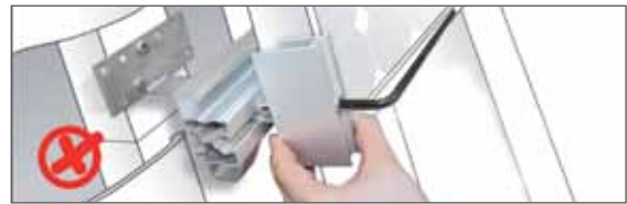
Do not use extended Allen keys!
