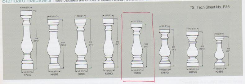
Non Standard Balusters Unless otherwise stated, these balusters are circular in section except top and bottom blocks which are square.
