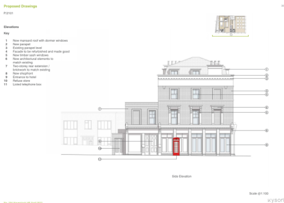
Drawing 1: As approved flank elevation showing the approved double doors and shopfront
