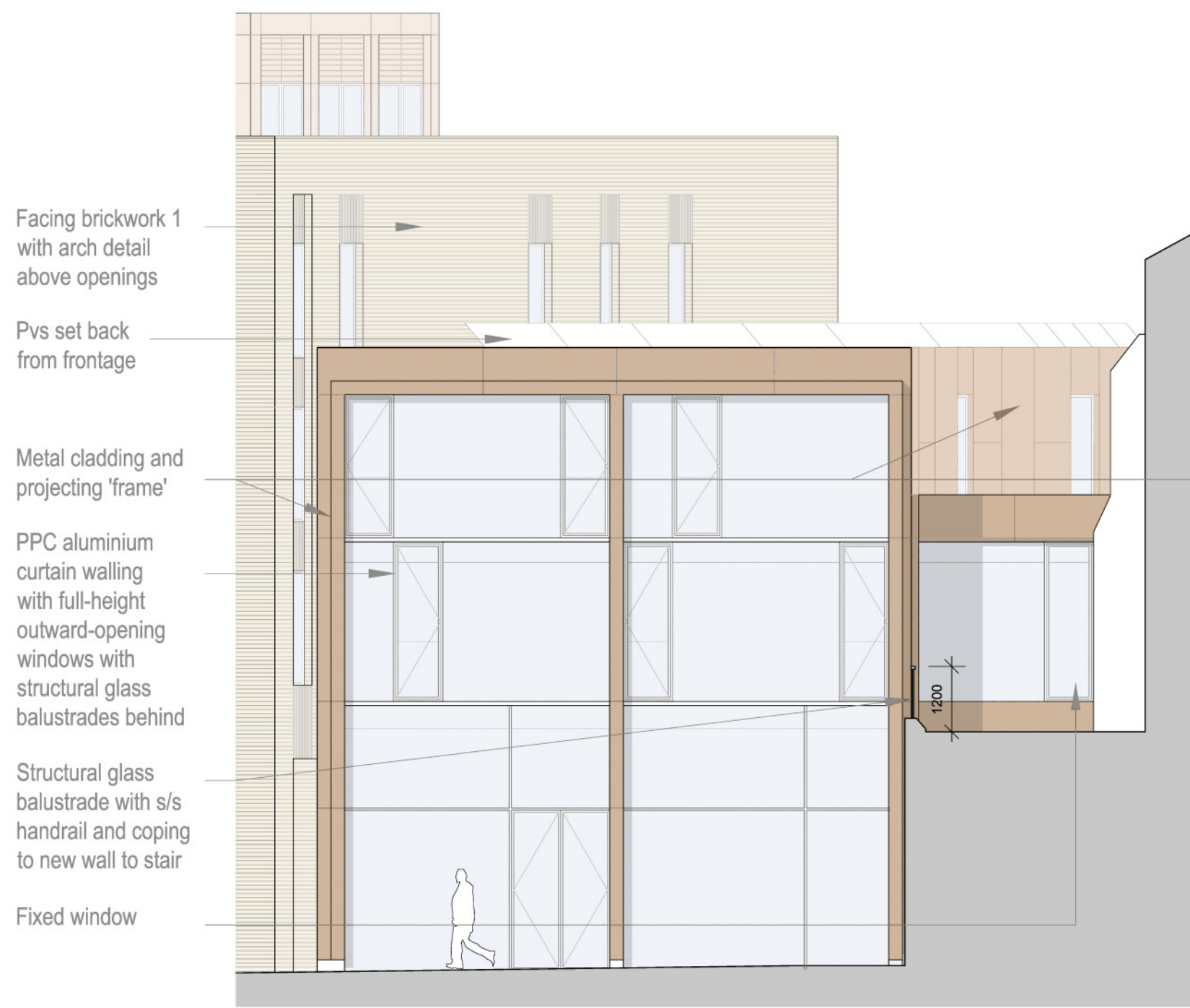
Detail North Elevation
