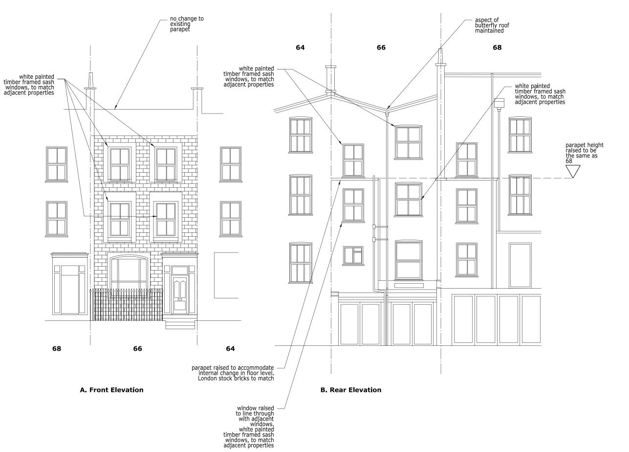
All drawings to be read in conjunction with structural engineer's and service engineer's Date 23.01.14 Note Planning Services Structures Mohsen & Ehsan Ghorani 66 Malden Road, Flat C Drawing Title **Proposed Elevation** Front & Rear Scale @ A3 1:100 Project No. Revision Drawing no. 2310 215 P1 Date of Issue Planning 23.01.14
