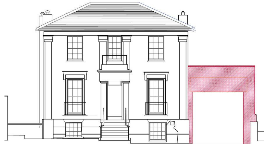
Fig. 4 Elevation of No1 Hawley Rd showing the existing annex No 1c Hawley Road (approved to be demolished) marked in red.
