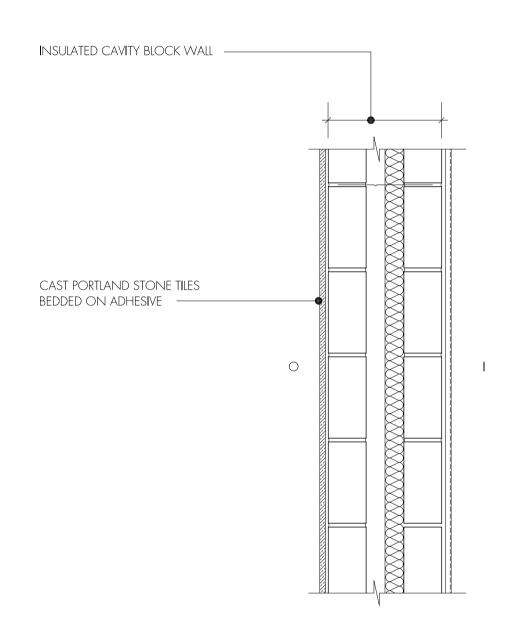
SECTION DETAIL OF STONE CLAD WALL 1:10
