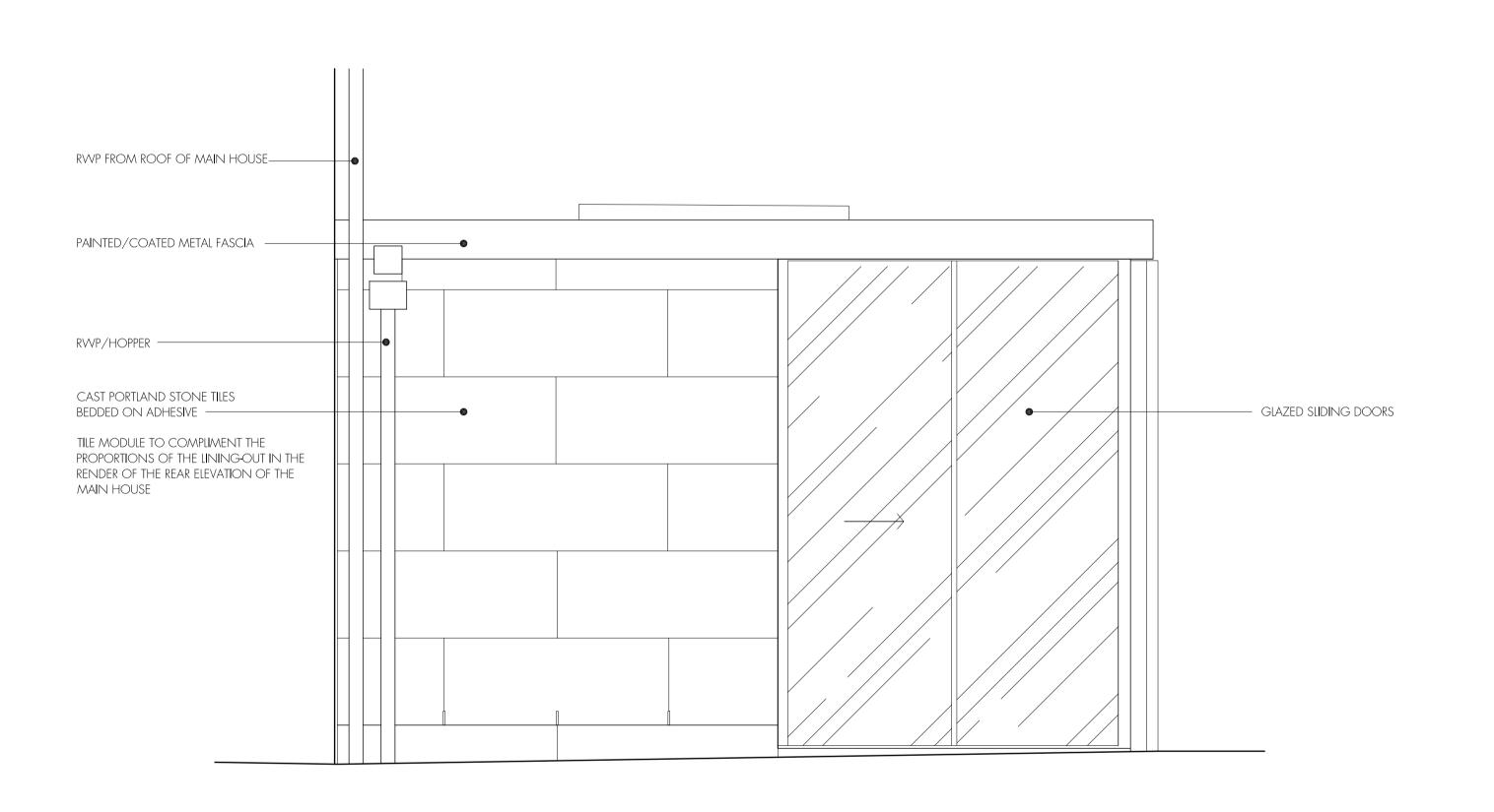
ELEVATION OF STONE CLAD WALL (REAR EXTENSION)
