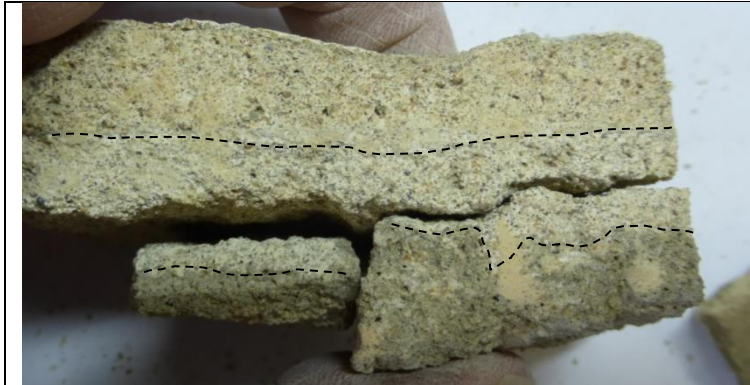
Plate 3. Sample S2 as received, with the sample reconstructed to show the top coat, intermediate coat and base coat. The coat interfaces are highlighted by broken lines superimposed onto the image.
