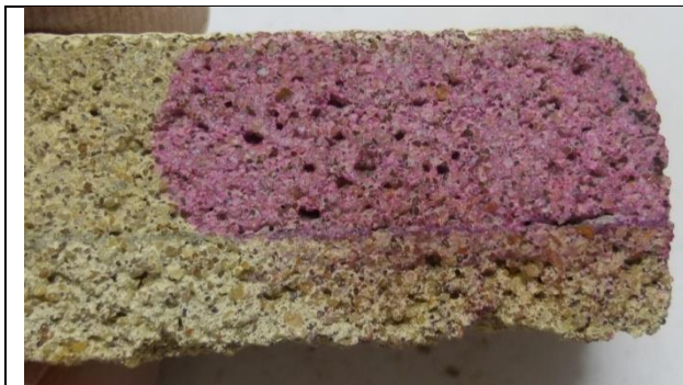
Plate 5. Finish coat tested with a droplet of phenolphthalein indicator solution, the fuchsia colour indicating that the mortar had not carbonated, except close to the outer surface.
