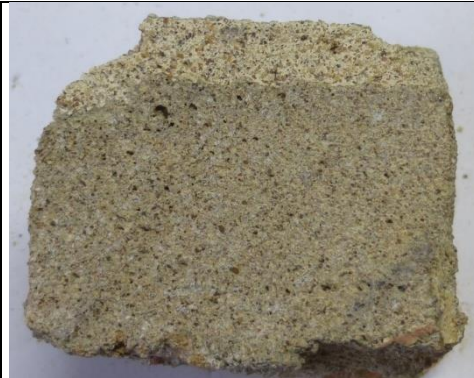
Plate 4. Separate sub-sample of the base coat with adhering intermediate coat on top. Again the intermediate coat appears to be a white cement mix, whereas the base coat is a grey OPC mix.
