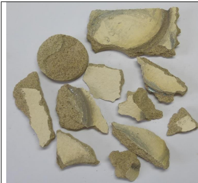
Plate 1. Sample S1 as received, with the sample consisting of several pieces of the finishing coat, with adhering paint finish on the outer surface and traces of the underlying intermediate coat adhering to its underside.
