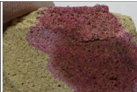
Plate 6. Phenolphthalein indicator test on intermediate coat and base coat again indicating no carbonation.
