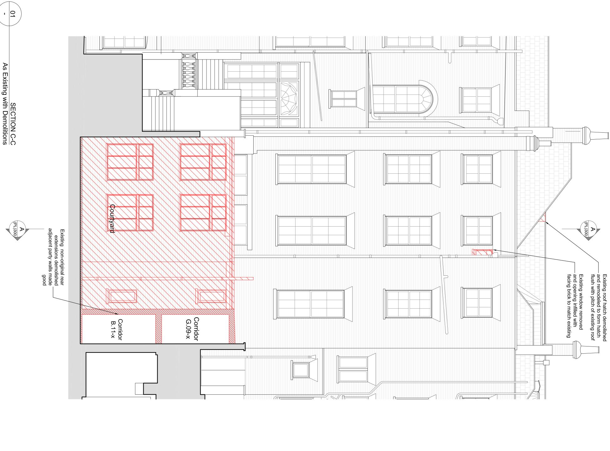
Where strengthening works to existing walls occurs, the ceiling below is to be made good and repaired to match existing. Refer to reflected ceiling plans for extents or repair works to ceilings.
