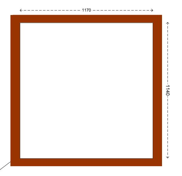
28mm Double Glazed unit Sealed 1170 mm x 1140 mm
