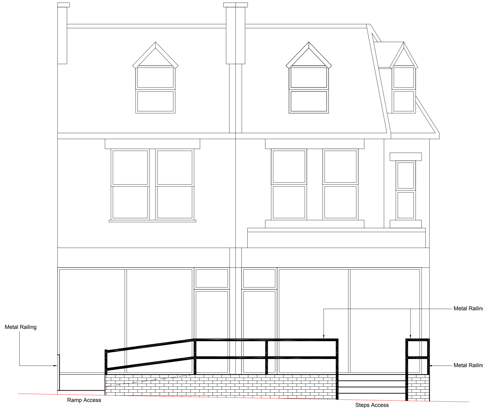
Proposed Front Elevation (Ramp) Scale 1:50
