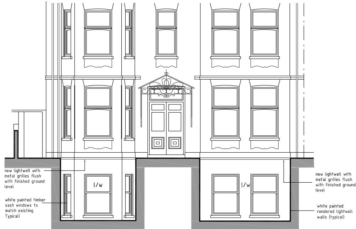
FRONT ELEVATION (AS PROPOSED)
