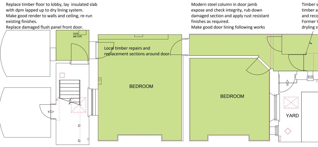
Modern Dry lining system removed. Carefully remove plugs and voids from walls. Make good brickwork and prepare for replacement dry lining system. Lift concrete slab, reduce levels and install integrated floor/wall drain system to dry lining.
