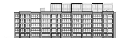
Six equal bays, each with a series of irregularly spaced zinc panels Frame around the bays so that the volume can be read as a single entity
