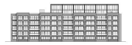
Finally, we opted for a slick, simple series of 6 equal bays, divided and sub-divided equally and with a zinc frame creating the appearance of a single entity. This fits in with the simple geometric forms below.
