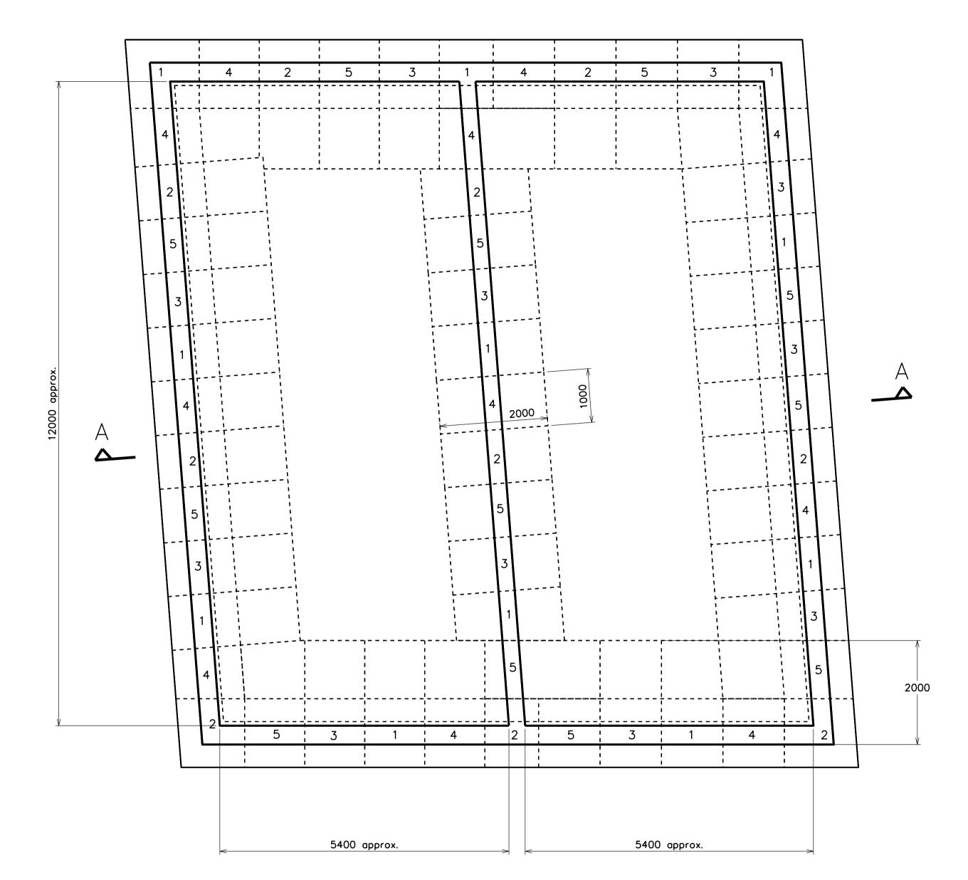
130 Holorib slab 130 Holorib slab 50 dry pack zone Typical. Projecting brickwork Dimension to match wall to be broken back flush with thickness but to be not Internal drainage layer (Delta or similar) less than 350 mm. wall face after underpinning applied to floor and wall surfaces is complete. 50 concrete blinding Mass concrete strip foundation centred on wall over 1200 1200
