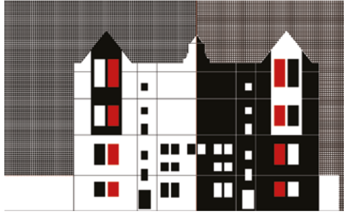
2. Fenestration There is a clear horizontal division of the main volume in four parts. Building components (e.g. windows) tend to be laid out in matching pairs.
