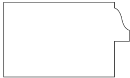
SECTION THROUGH SASH & CASEMENT STYLES scale 1:1 @ A1 & 1:2 @ A3
