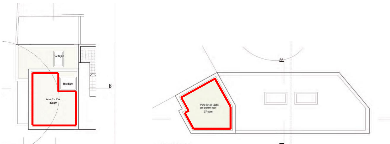
Available Roof Area for PVs (site 1 = 33m 2 , site 3 = 27m 2 )
