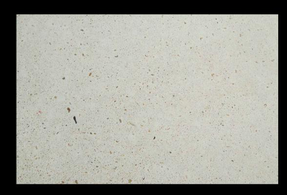
Sandwich Street Main Building: Cast Stone Cast stone to all sills, soffits and stone facades with an aggregate mix of wet-cast concrete mix of Cotswold gravel and a 50%:50% mix of Cotswold and Dolomite sands and white cement with an acid etched surface finis h
