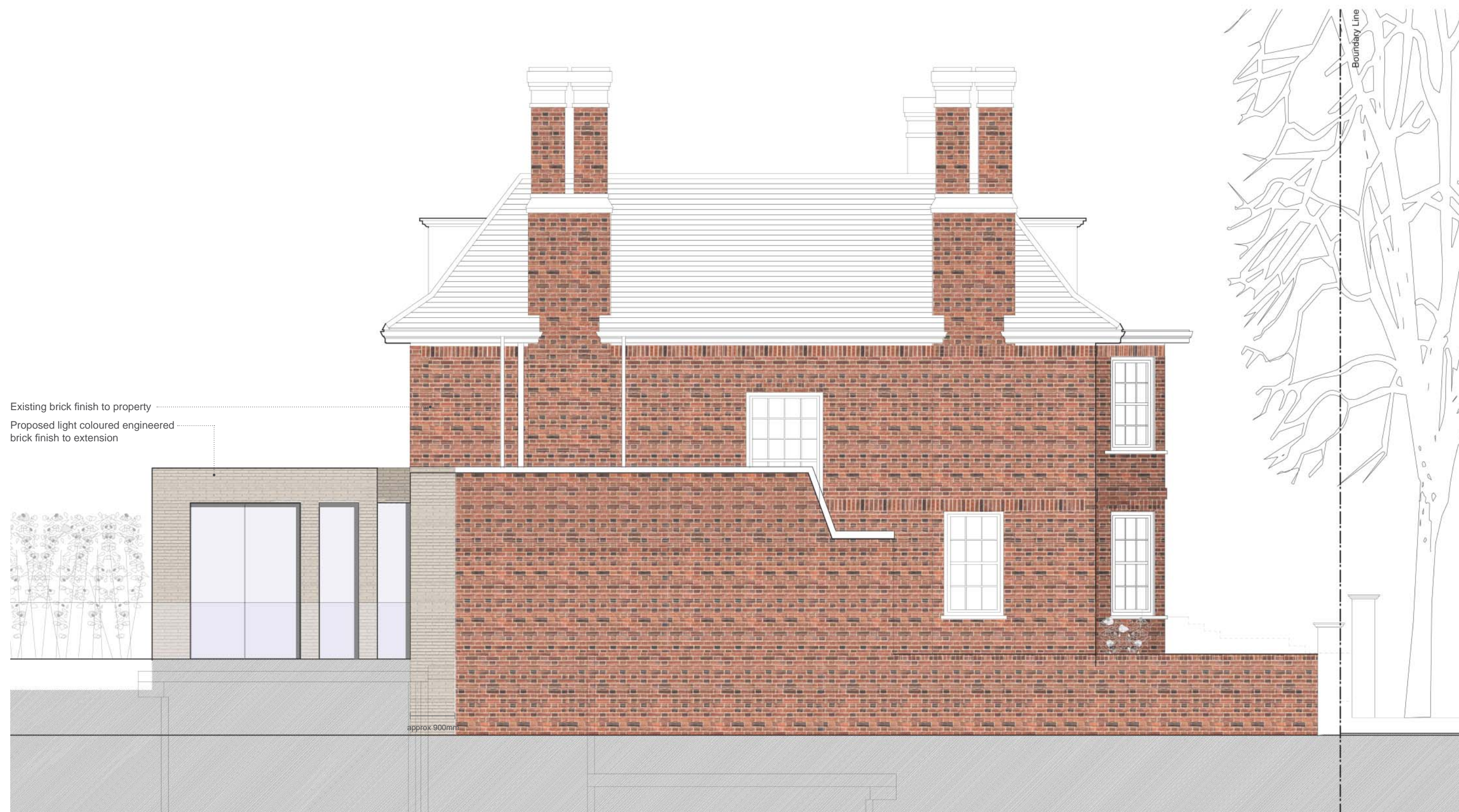
236-02(A) - SIDE ELEVATION (TO NO.61) - Light Coloured Brickwork to proposed extension Proposed amendment to Planning Ref: 2013/0825/P | 63 Frognal, London, NW3 6YA
