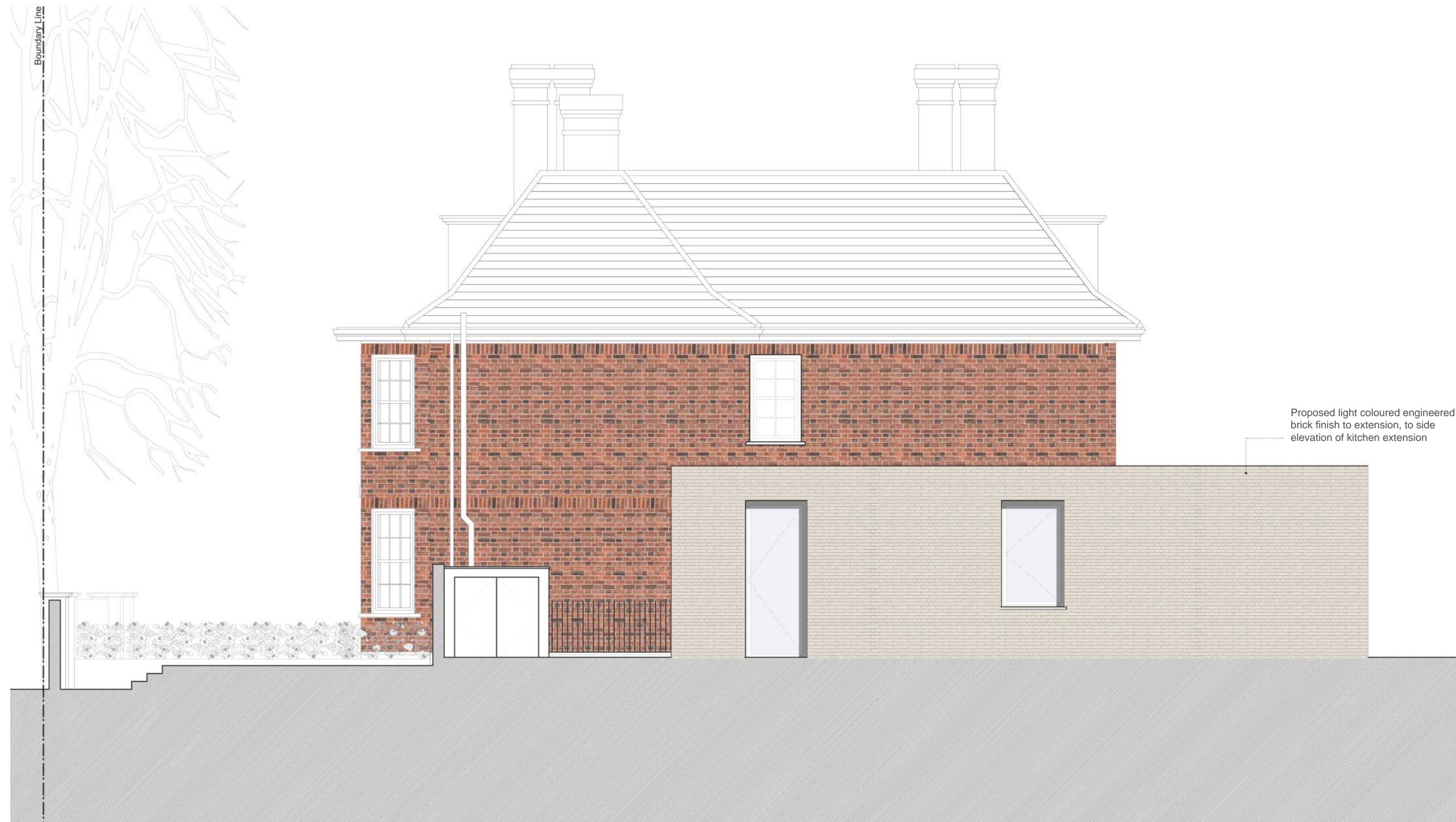
236-03(A) - SIDE ELEVATION (TO NO.65) - Light Coloured Brickwork to proposed extension Proposed amendment to Planning Ref: 2013/0825/P | 63 Frognal, London, NW3 6YA
