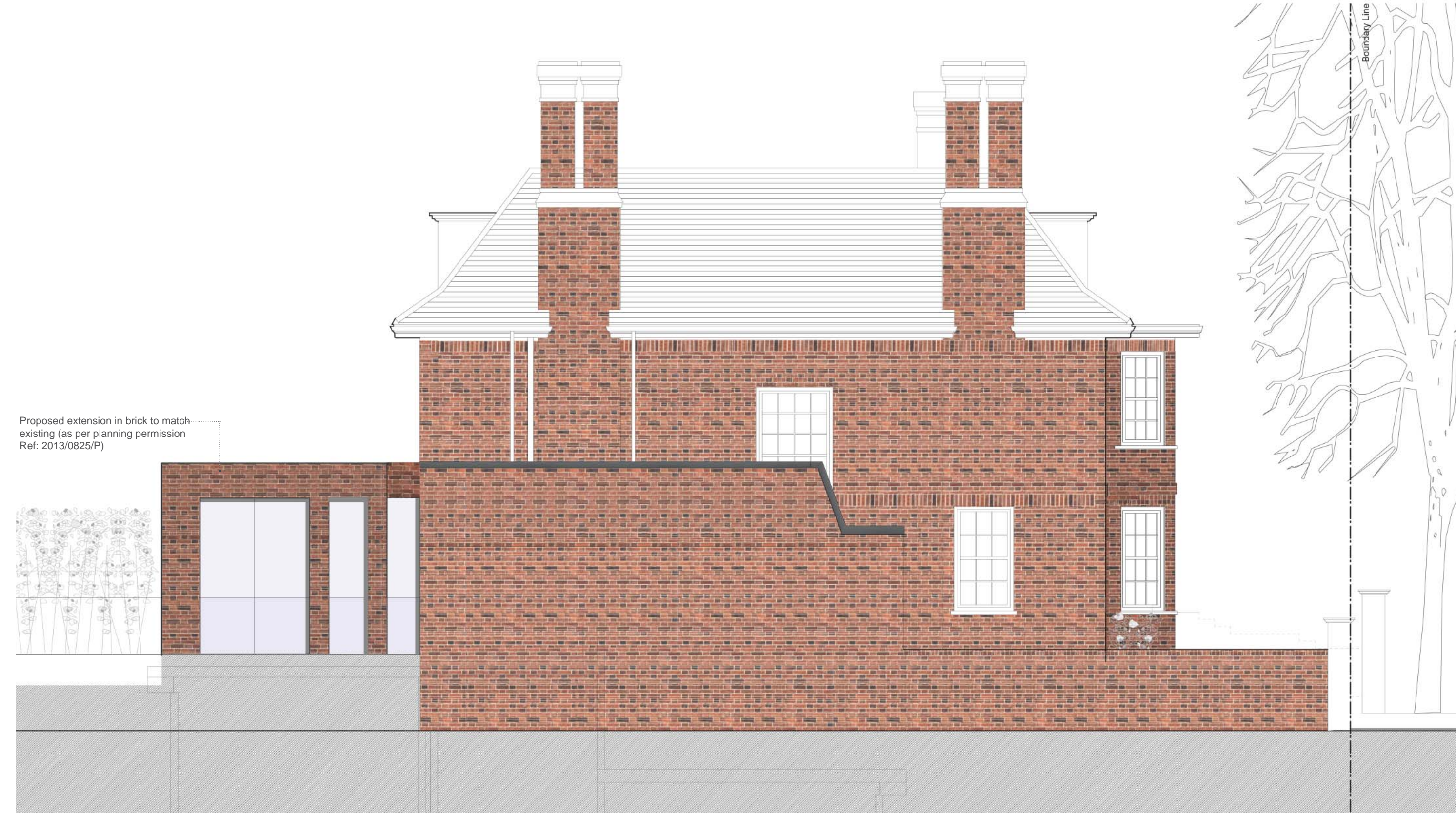
236-02(B) - SIDE ELEVATION (TO NO.61) - Brickwork to match existing As per Planning Ref: 2013/0825/P | 63 Frognal, London, NW3 6YA
