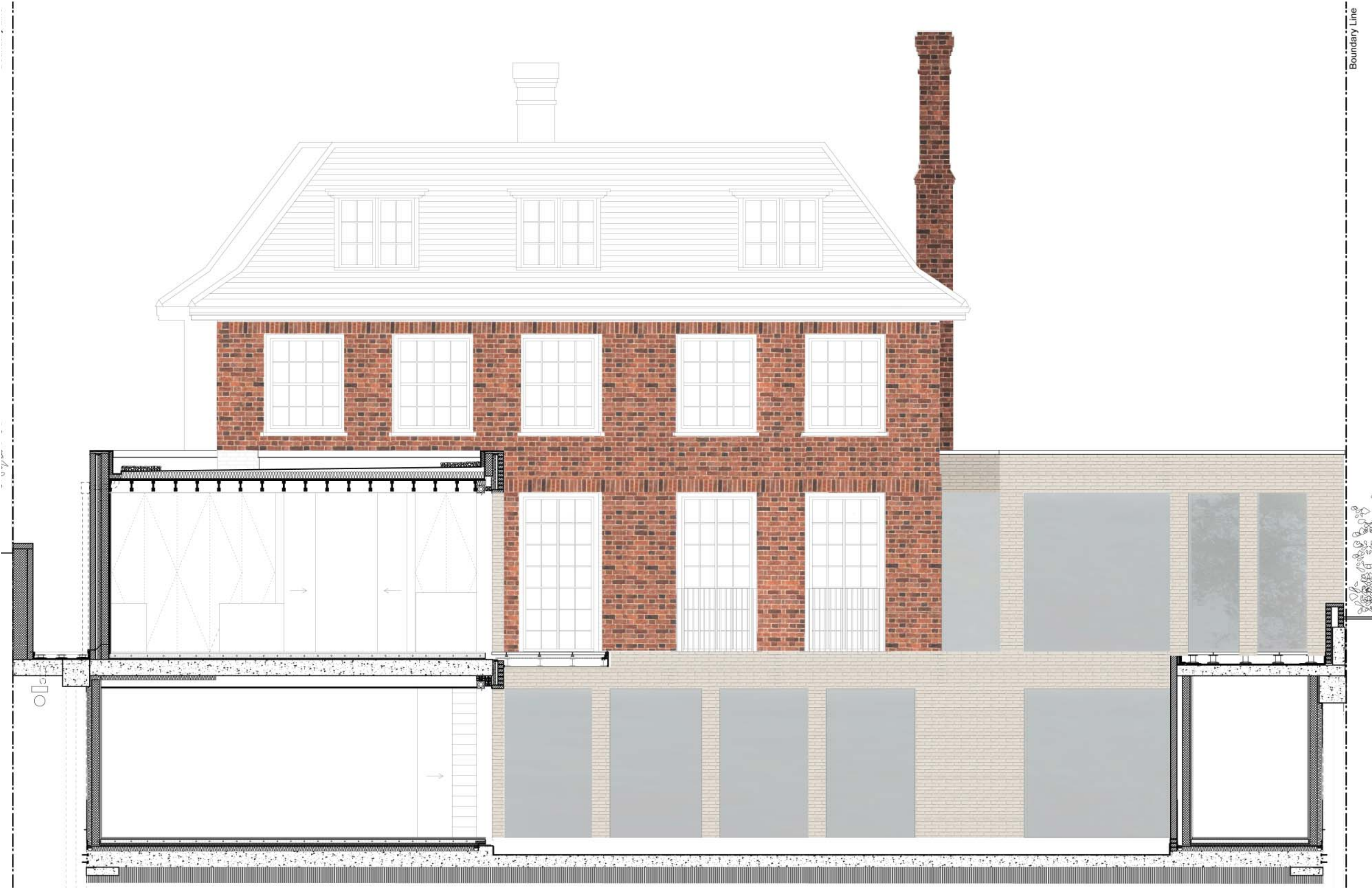
236-04(A) - REAR ELEVATION/SECTION - Light Coloured Brickwork to proposed extension Proposed amendment to Planning Ref: 2013/0825/P | 63 Frognal, London, NW3 6YA
