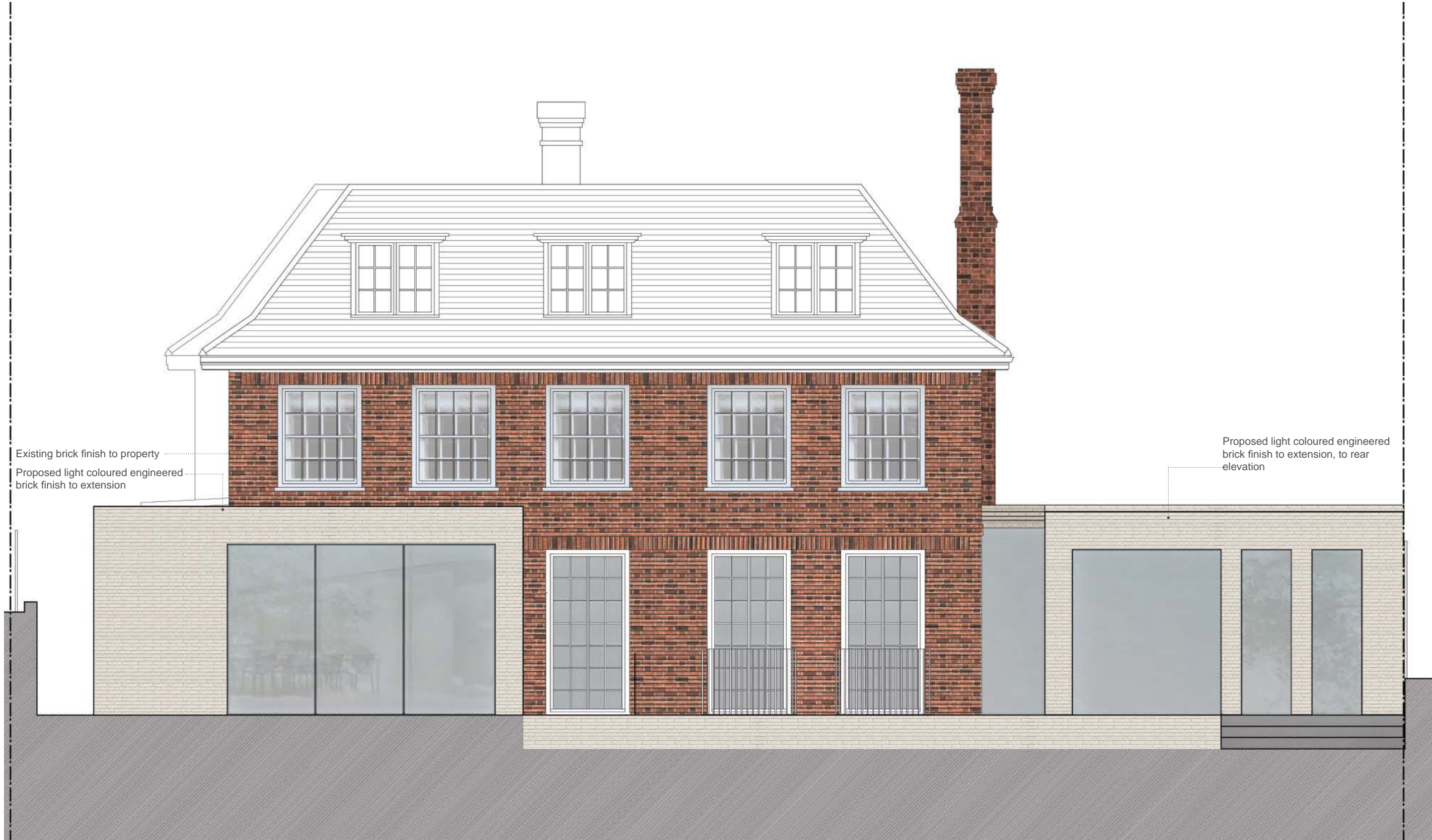
236-01 (A) - REAR ELEVATION - Light Coloured Brickwork to proposed extension Proposed amendment to Planning Ref: 2013/0825/P | 63 Frognal, London, NW3 6YA
