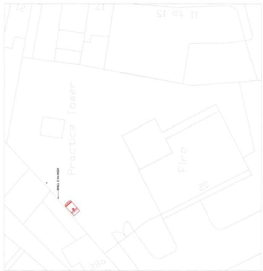
PROPOSED: NEW 5000LTS DERV ABOVE GROUND FUEL TANK SCALE 1:250
