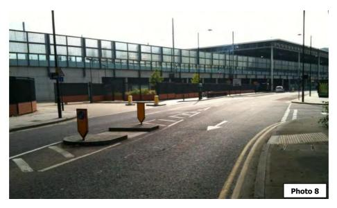
1.21 As can be seen from **Photo 8** the informal crossings provide dropped kerbs and tactile paving of the appropriate colour. The central refuge is level with the carriageway to assist mobility impaired users and provides sufficient crossing capacity.
