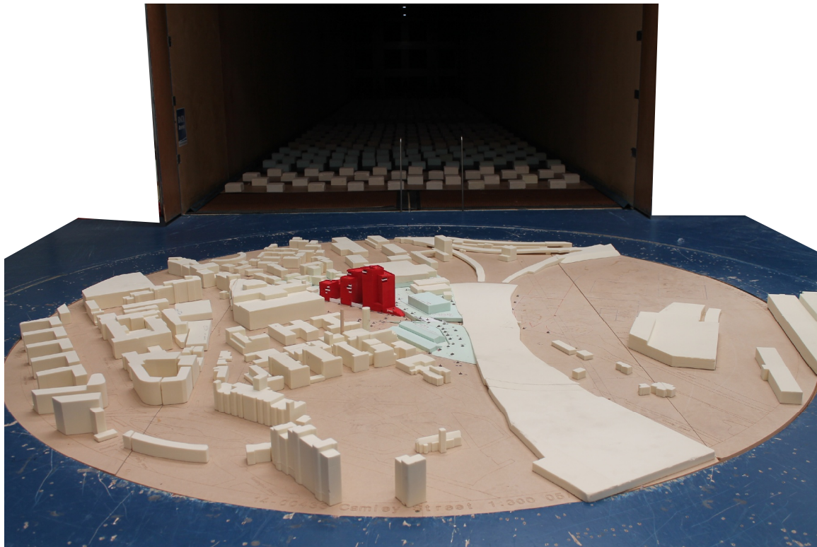
Figure 11: Current Site and Existing Surroundings including 103 Camley St (Configuration 1) – View in the Wind Tunnel (view from south)
