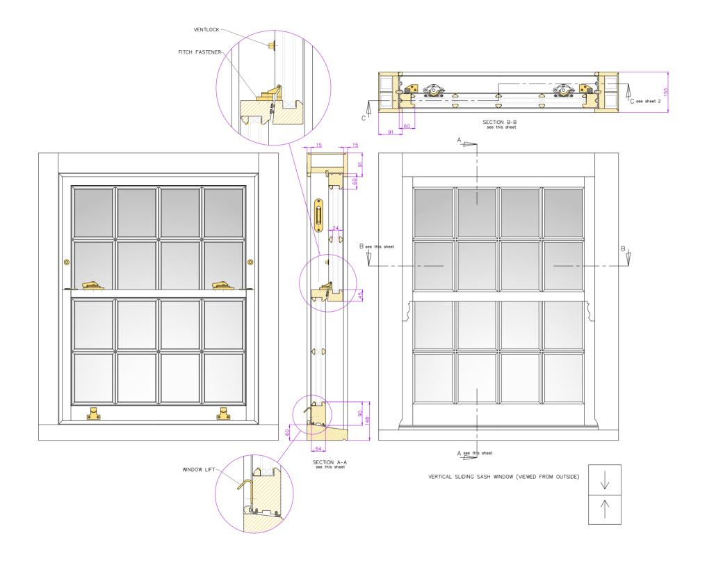
TYPICAL REPLACEMENT TIMBER SASH WINDOW DETAILS TO FRONT AND REAR OF THE PROPERTY. REFER TO DRAWINGS P001-P004 FOR LOCATION AND TYPE OF WINDOW SPECIFIED. PROPOSED REPLACEMENT WINDOWS DO NOT INCLUDE SASH WINDOW BARS AS SHOWN.
