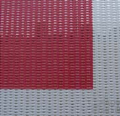
Mesh banner material allows air to flow through, reducing wind load by up to 50%
