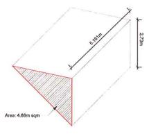
The volume of the roof has been calculated as 4.86 sqm x 5.16 m to equal: 25.08 cubic metres
