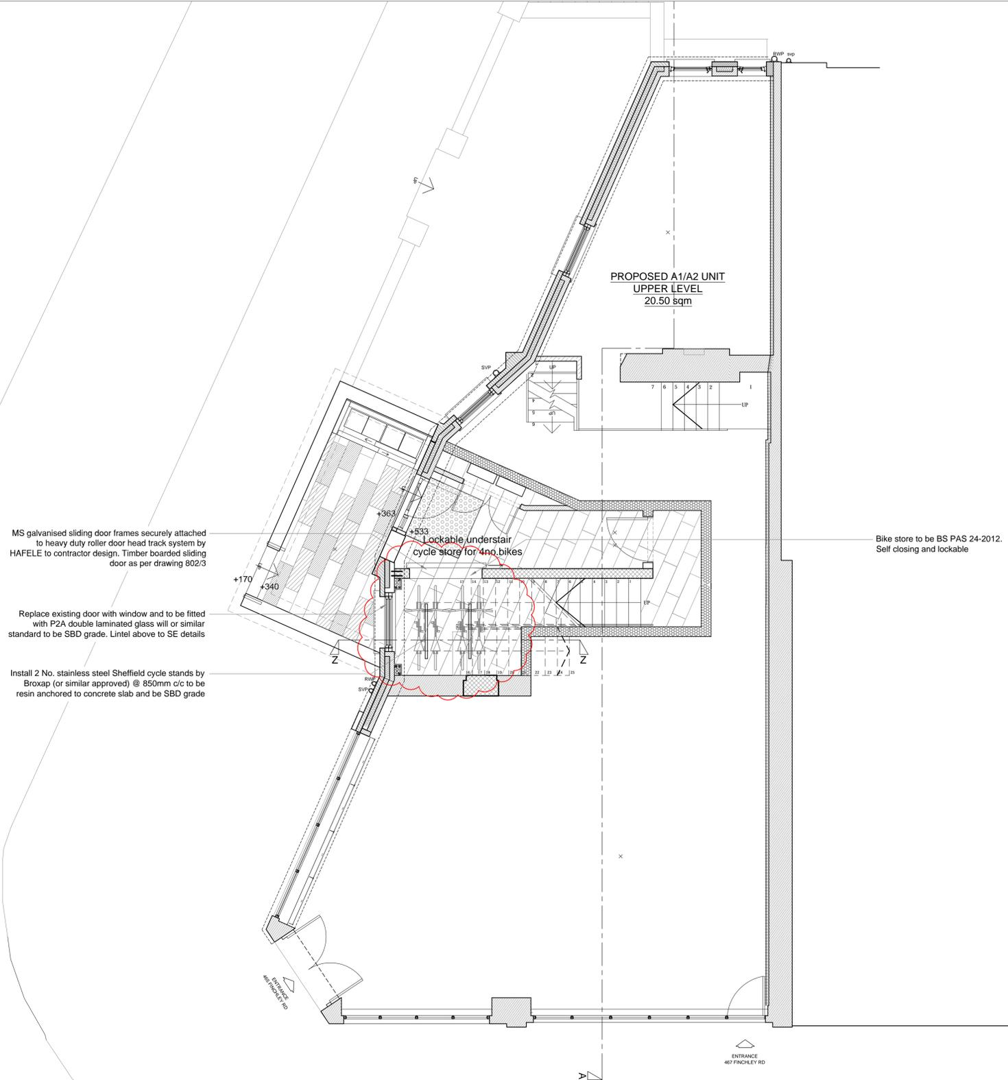
1 Proposed Ground Floor Plan showing cycle storage to upper parts
