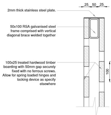
3 Typical timber gates construction (plan)
