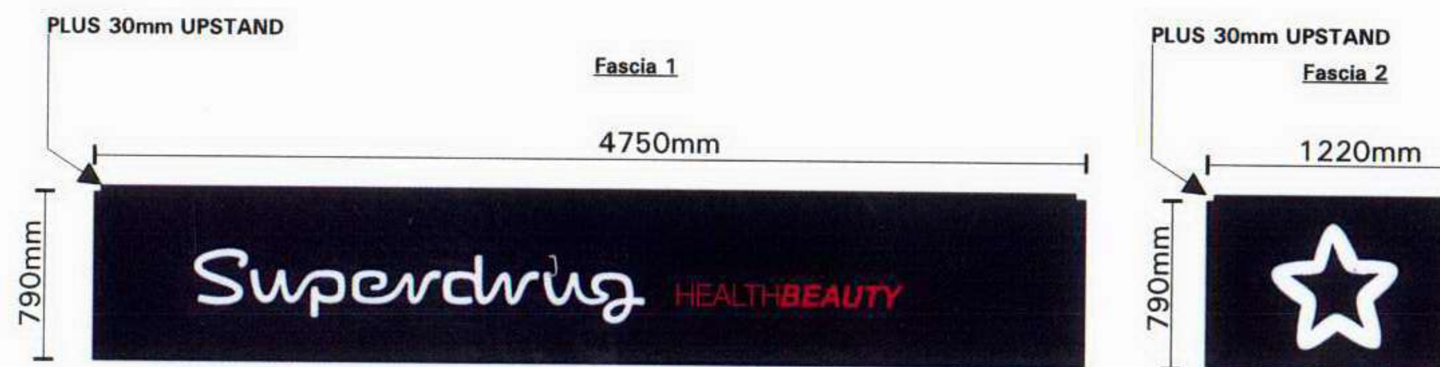
INTERNALLY ILLUMINATED FASCIAS. Scale 1:50
