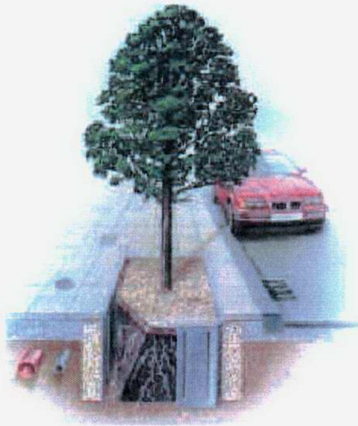
Fig. 1: Shows confined tree pit direct roots down with root barriers. This form of planting can be extended in length to accommodate numerous trees in one trench.
