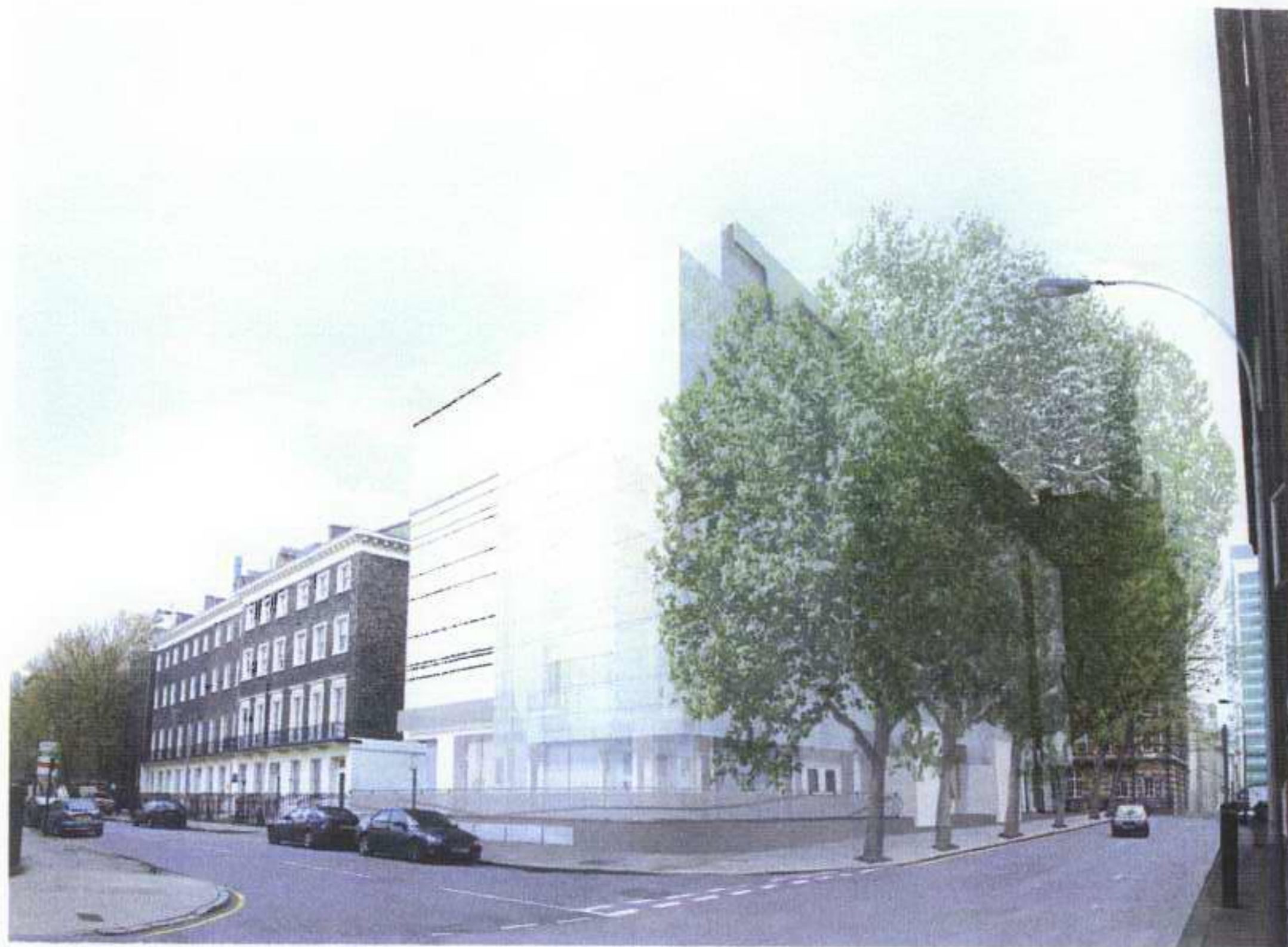
Figure 9. View at junction of Taviton Street & Endsleigh Gardens: current Planning Submission showing rendered façade with horizontal banding adjacent to existing houses.
