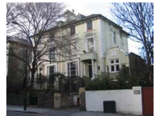
Italianate Semi Detached Villa. Painted render, generous fenestration, vertical proportions, designed to be viewed from the corner, side walls not blank.
