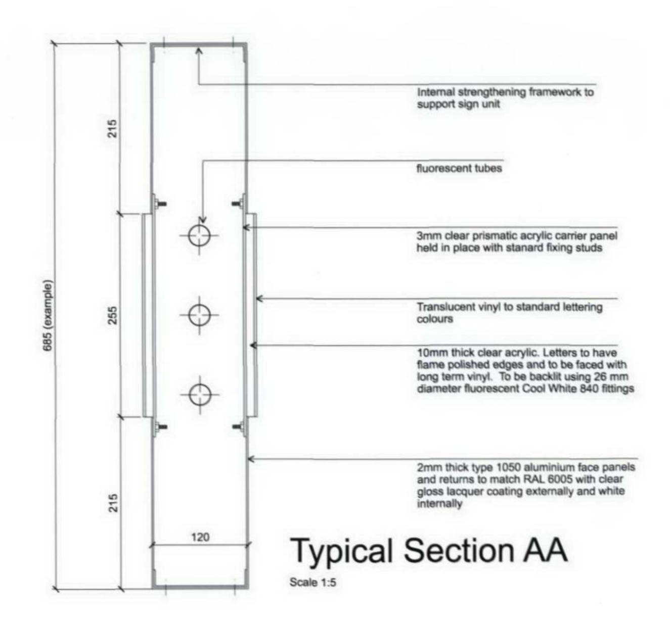
Sign B3 - Typical Double Sided Projecting Bus Stop Sign (Internally illuminated box sign)
