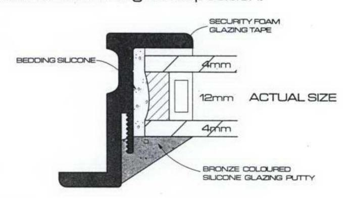
The glass can either be finally sealed in with a bronze coloured silicone or glazing putty.
